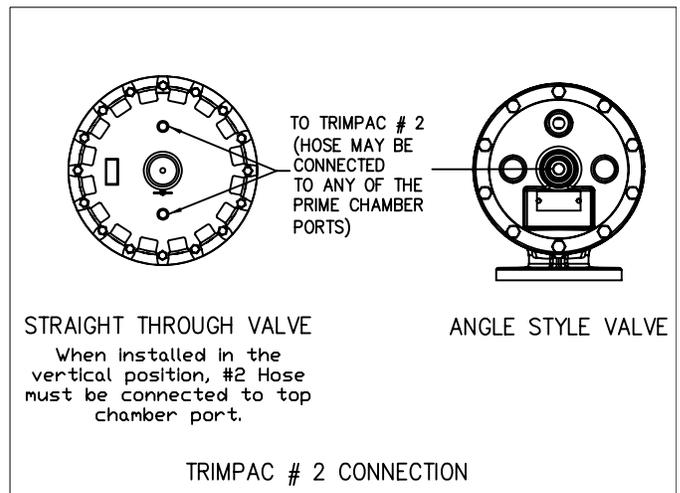
**Figure 11 - Valve Connections**
